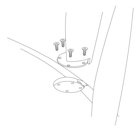
Screw four short screws for each leg. Repeat the process until all four legs are fixed to the table top. (TIP: Wait until all four screws are partially fixed to the table top before tightening them.)
